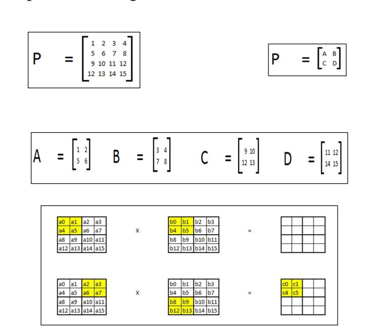
In this project the base block for matrix multiplication is considered as 4x4 which is implemented on the hardware.
