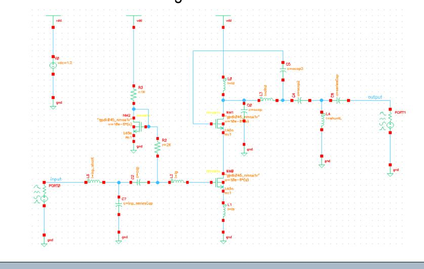
S11 reflects the input matching of the LNA (input reflection coefficient). We were able to achieve approximately -18dB for return loss. The lumped T matching network at the input was carefully tuned to achieve this result.
