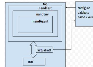
The performance monitor is designed to monitor the performance of the NAND Flash controller and it monitor the number of cycles taken by the NAND flash controller during burst write and burst read operation. It also monitors the total number of cycles taken by the controller for individual read and the page program operation.
