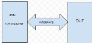
Main task of UVM verification environment is to generate stimulus which are given to the DUT and monitor the response coming from the DUT. Design under test consist of two main parts: NAND flash controller and NAND flash memory and there is one bus master which is used to connect memory and controller and it is responsible for handling the different read, write, read Id transactions.[2]
