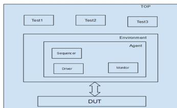
UVM environment is implemented using the components shown above in the figure. Once the base of verification environment is set and all the components are placed in proper hierarchy and well connected same environment can be used for different tests [3].
