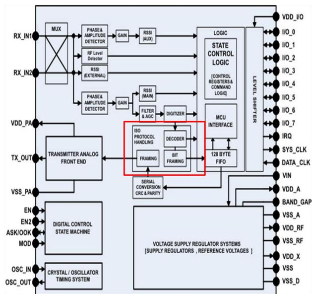
This system included a PCD module(reader), Manchester encoder module for sending secure data to the tag. It also includes a PICC module(tag) and Modified Miller encoder to encode the baseband signal.
