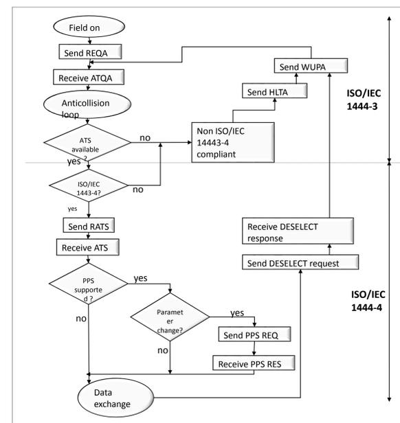
The design implements the above flow which is a reference to the standard and covers the complete process of selecting a particular PICC and data exchange.
