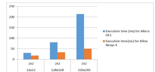
Above graph shows the comparison of processing time for Altera and Xilinx FPGA platforms for different image size.
