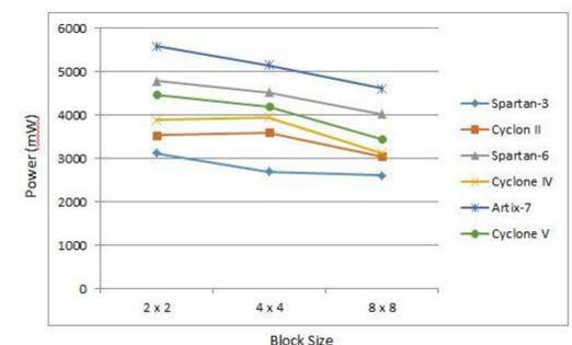
For equivalent FPGA configuration, Altera FPGA development board performs faster than Xilinx FPGA board (except Spartan 6) and also consumes less power.
